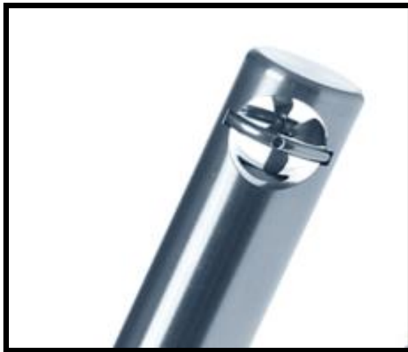
Figure 3-17. Vane anemometer wheel [11]
