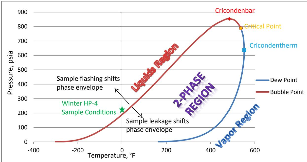
Figure 2-6. Phase envelope for a PHLSA Study condensate sample.
