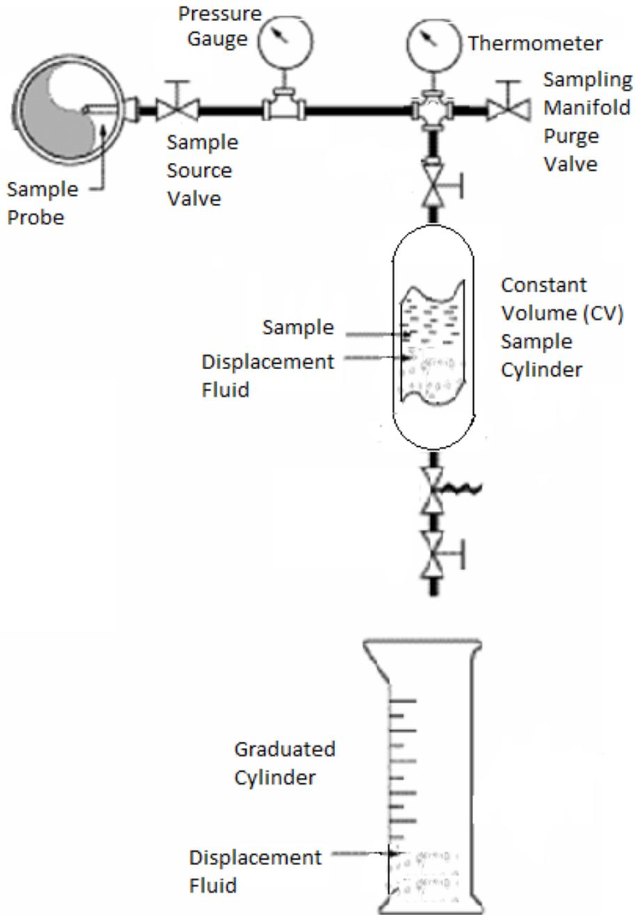
Figure 2-4. Constant volume cylinder using water displacement with sampling system manifold.
