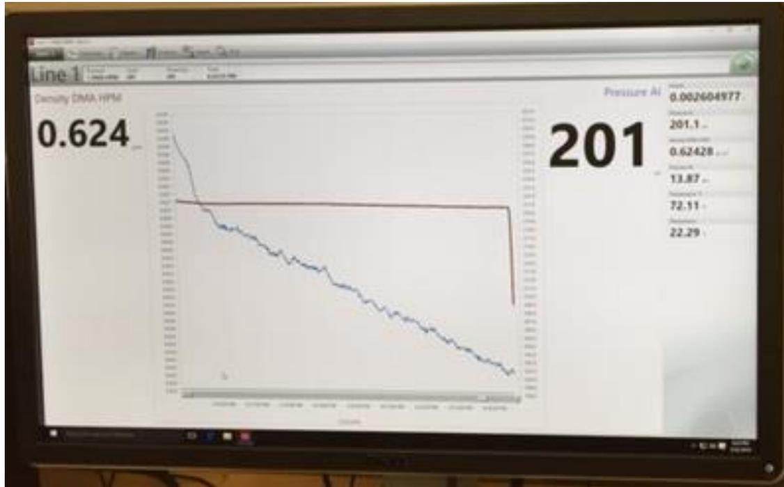
Figure 2-5. Pressurized densitometer bubble point determination.
