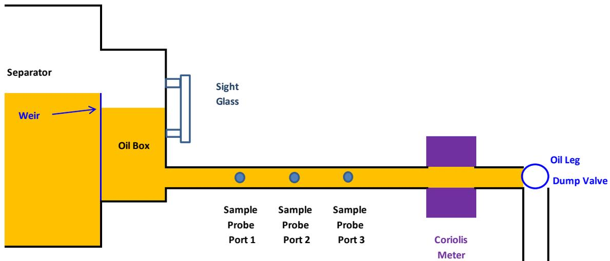
Figure 3-1. Sample probes and sight glass sample collection location schematic.
