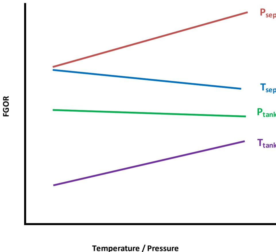
Figure 2-2. Impact of separator and tank pressures and temperatures on flash gas generation.
