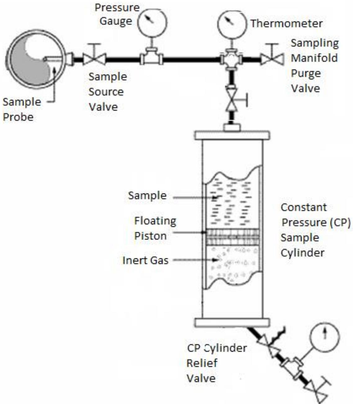
Figure 2-3. Floating piston/constant pressure cylinder sampling system with sampling manifold.
