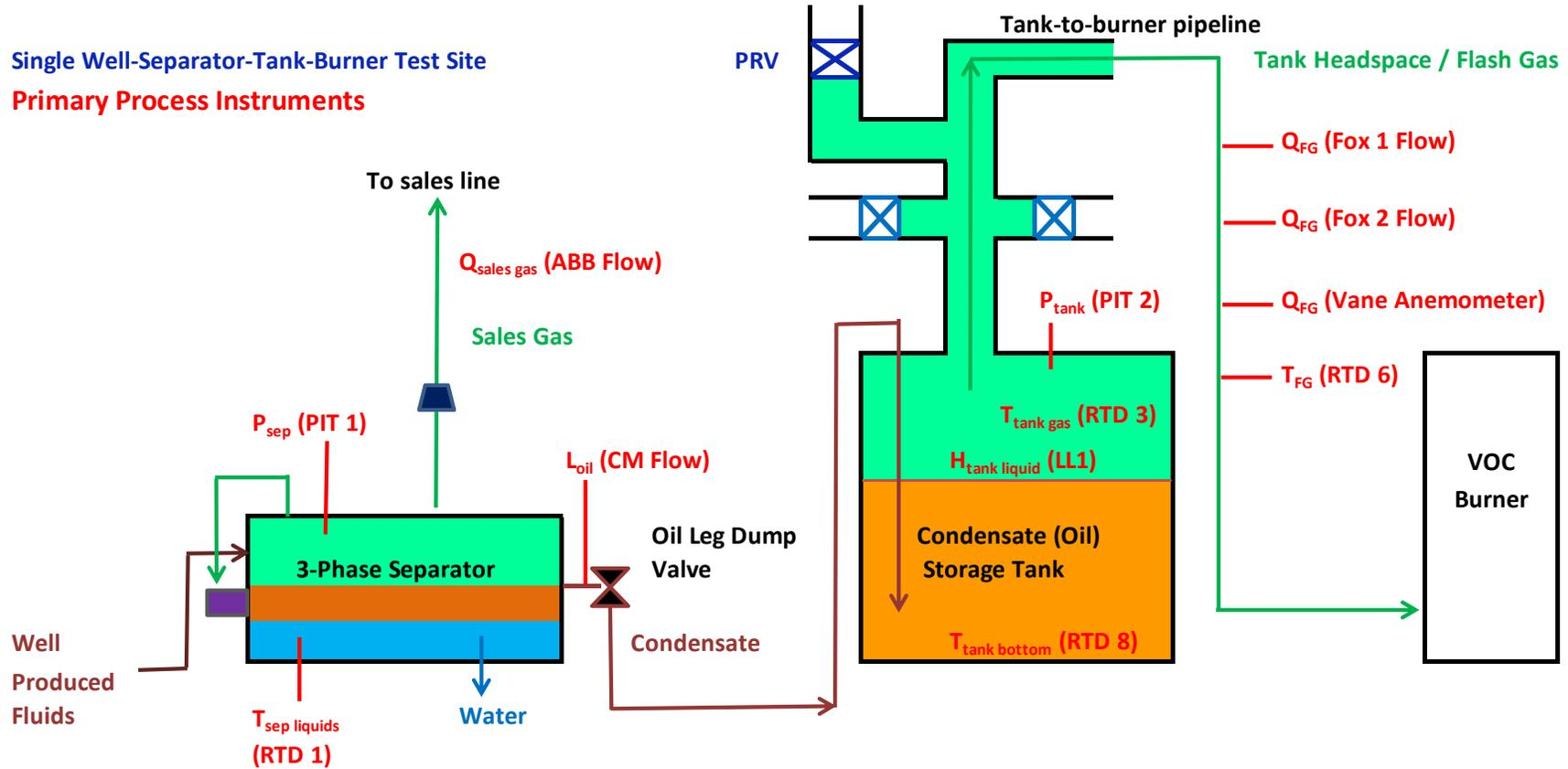
Figure 3-2. Primary process measurements during three-pressure testing.
